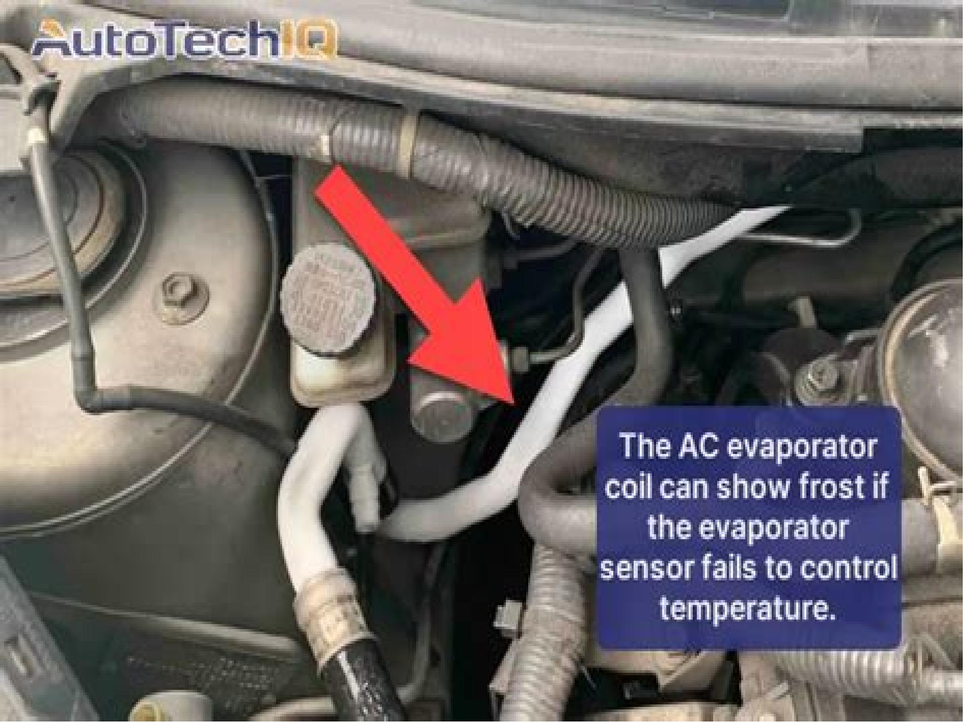
The AC evaporator coil can show frost if the evaporator sensor fails to control temperature.
